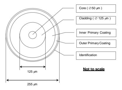
Fig. 1 Cross Section View of Multimode Fiber (50/125, Graded-index)
